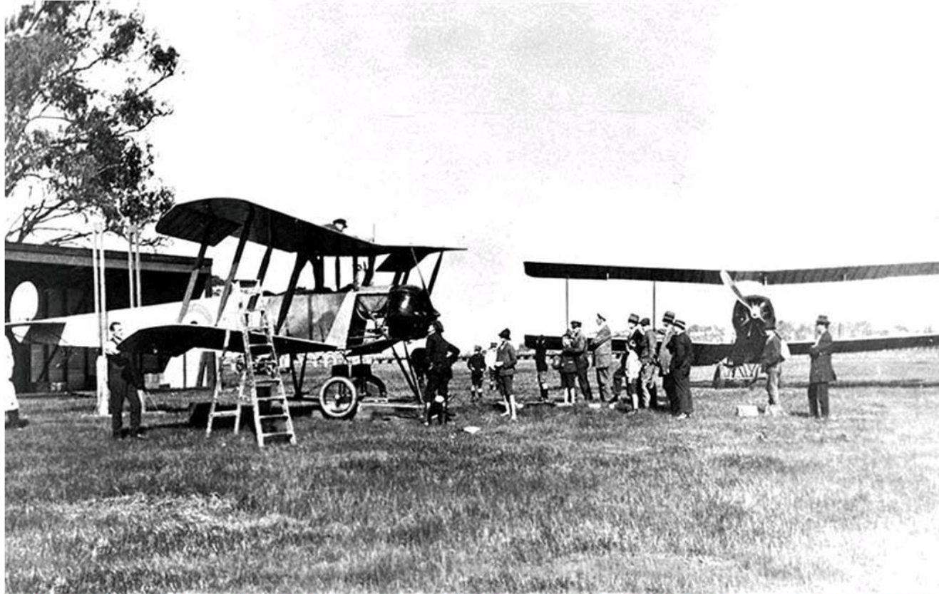
Major Norman Brearley's two Avro 504Js were shipped to Fremantle on board the Port Napier, arriving in July 1919. Here they are being assembled at the Belmont Racecourse in Perth at the end of that month. Both were powered by 100hp Gnome Monosoupapes rotary engines
