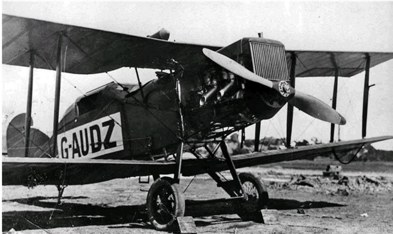
G-AUDZ on completion at Maylands with the WAA-designed horn-balanced rudder which was fitted to all the Bristols
