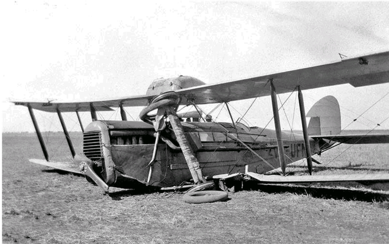
VH-UFN at Noonkanbah Station in the Kimberleys September 1931, after a tyre burst on landing causing a severe ground-loop.
