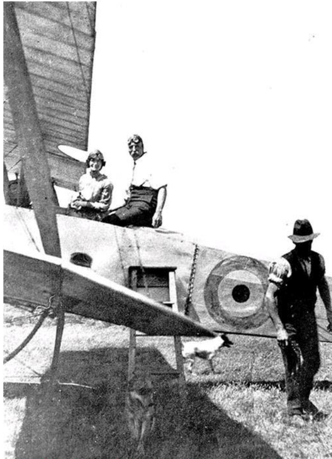
Joyriding scene with the farm dog taking advantage of the shade under the Avro. Note the stitching in the fuselage fabric
