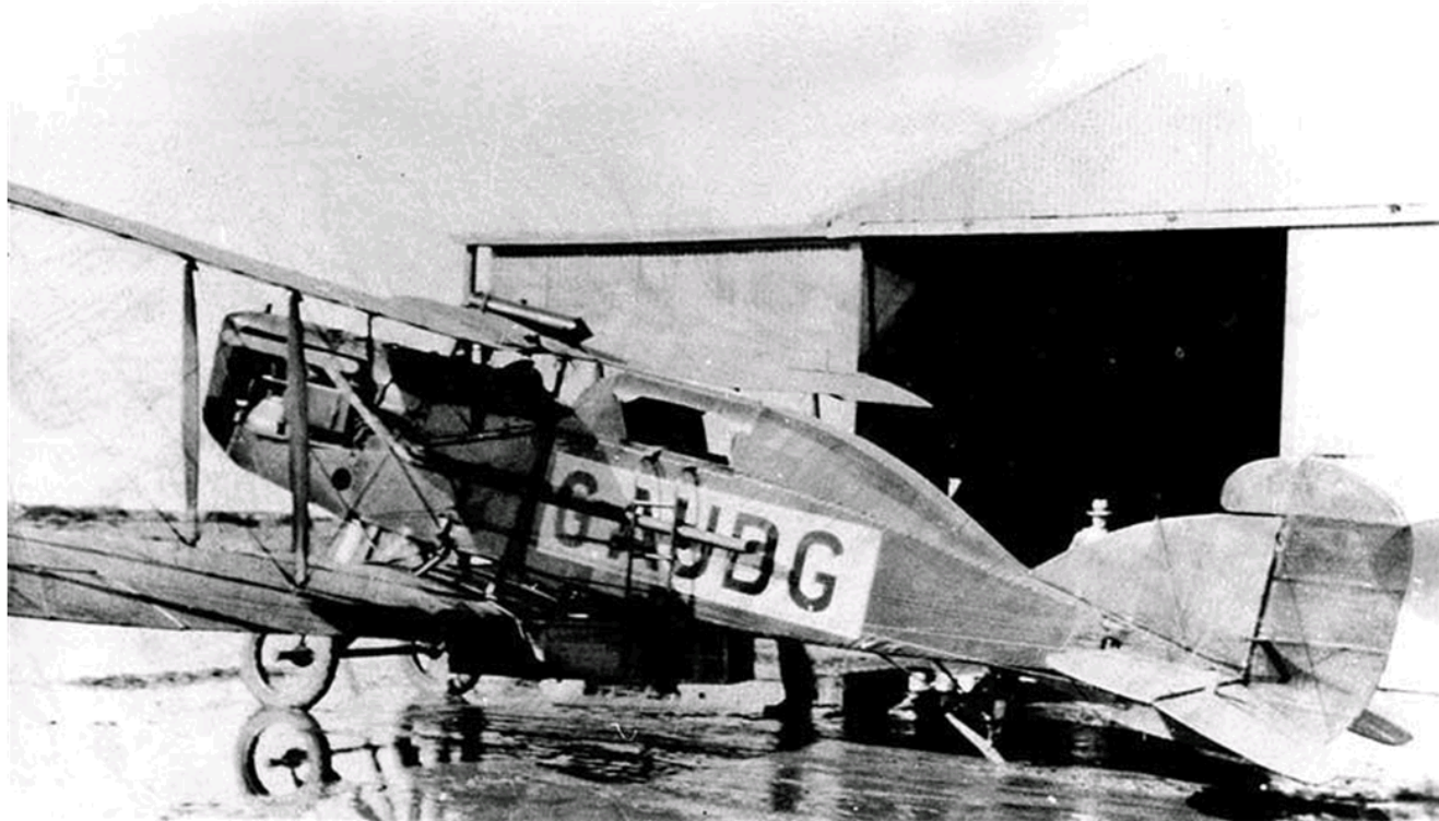
The metal box attached under the fuselage carried supplies and tools. It was referred to by WAA staff as the "Gubbins Box". Photo: The Collection
